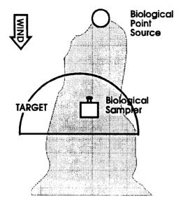
Figure 5-15a. Correct Placement of Sampler.
